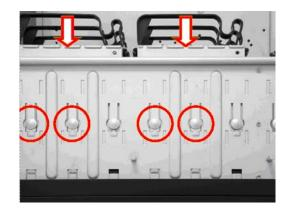
First press the two round shape button using your thumbs, then use your index finger to push the middle 3.5" module to remove it.
